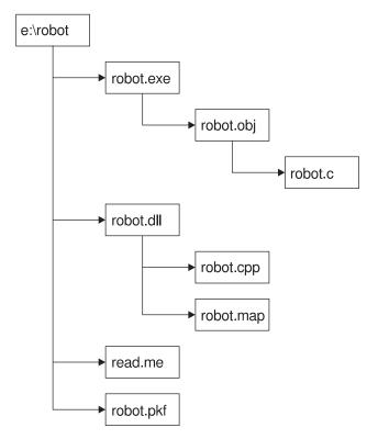
Figure 68. Adding the gather step to the build tree
